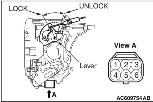
**STEP 15. Check the rear door lock actuator (LH).**
