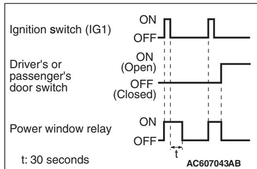
Even after the ignition is switched off, the ETACS-ECU keeps the power window relay activated for approximately 30 seconds, enabling raising or lowering of the power windows by using the power window switches. After approximately 30 seconds, the power window relay is deactivated. During this timed operation, if the driver's or passenger's doors are opened, the power window relay is deactivated from that moment.
