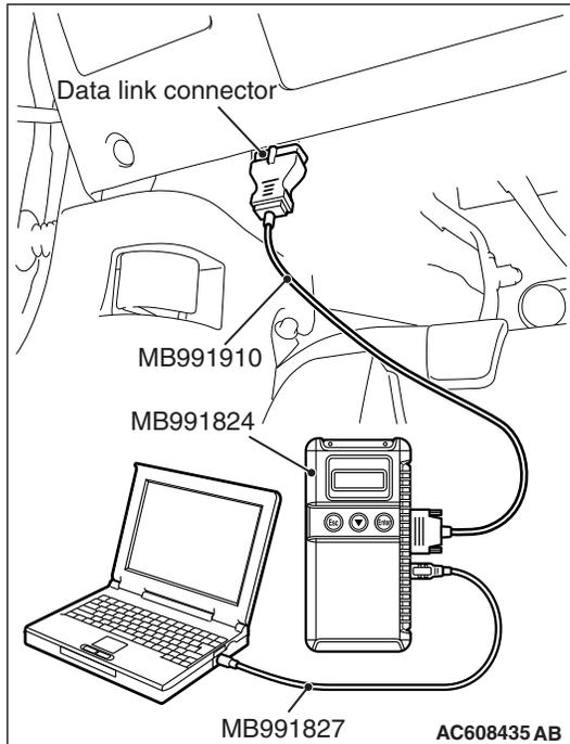
**STEP 3.** Using scan tool MB991958, read the diagnostic trouble code.
