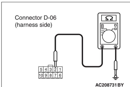
**STEP 10. Check the wiring harness between sunroof motor assembly connector D-06 (terminal 2) and ground.**
