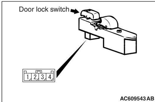
**STEP 3. Check the front power window sub switch (door lock switch).**
