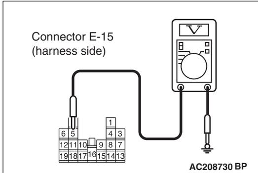
**STEP 11. Check the ETACS-ECU connector C-315 line circuit to the power window main switch. Measure the voltage at power window main switch connector E-15.**
