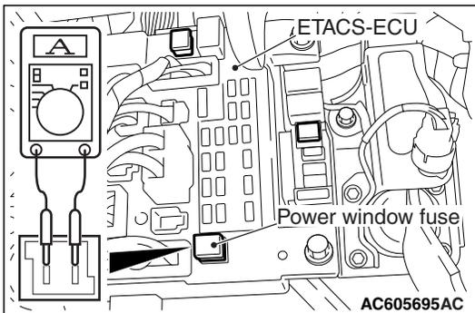
1. Remove the power window fuse, and connect a multimeter as shown in the illustration.
