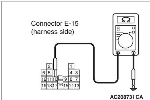
**STEP 14. Check the ground circuit to the power window main switch. Measure the resistance at power window main switch connector E-15.**
