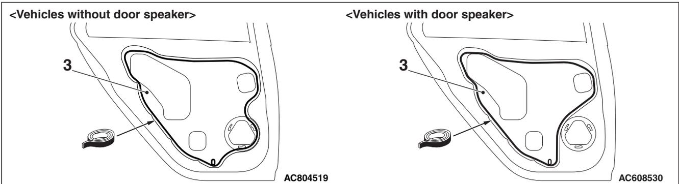
Sealant: 3M™ AAD Part No.8633 or equivalent
