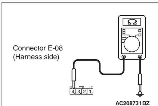
**STEP 4. Check the ground circuit to the front power window sub switch. Measure the resistance at front power window sub switch connector E-08.**
