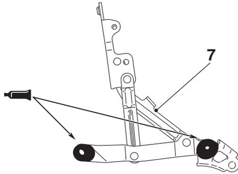
ADHESIVE: 3M AAD PART NO.8531 HEAVY DRIP CHECK SEALER, 3M AAD PART NO.8646 AUTOMOTIVE JOINT AND SEAM SEALER OR EQUIVALENT
