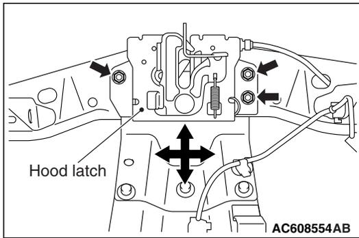
2. Loosen the hood latch mounting bolts but do not remove them. Move the hood latch up/down and left/right to align the hood level and adjust the hood striker engagement.
