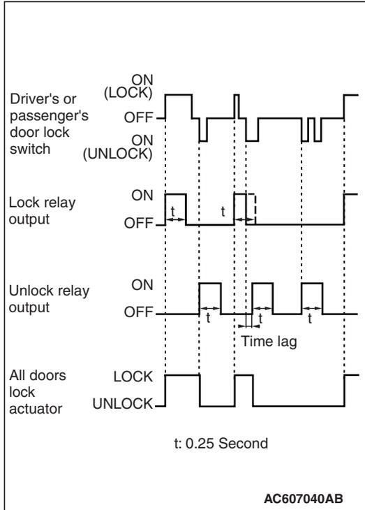
When the door is locked by the driver's or passenger's door lock switch, the ETACS-ECU operates its door lock relay and passes a current through the door lock actuators of all the doors for 0.25 second to lock all the doors.
