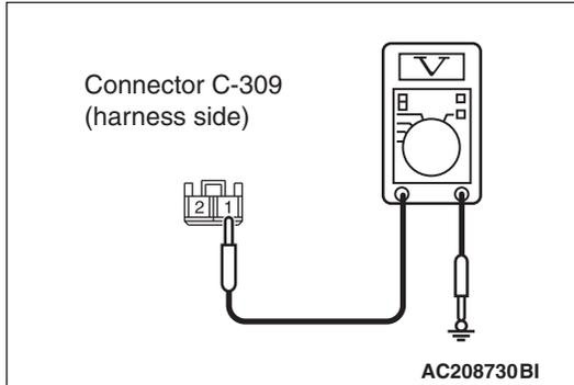
**STEP 5. Check the fusible link (34) line of power supply circuit to the ETACS-ECU. Measure the voltage at ETACS-ECU connector C-309.**
