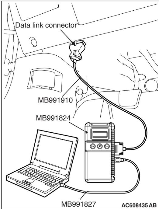
**STEP 4. Using scan tool MB991958, check data list.**
