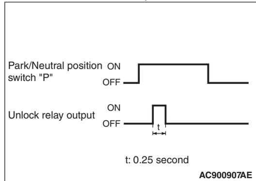
When the selector lever is shifted to the P position with the ignition switch turned ON, the lever position sensor "P" turns ON, ETACS-ECU turns the unlock relay output ON for 0.25 second to unlock all the doors.
