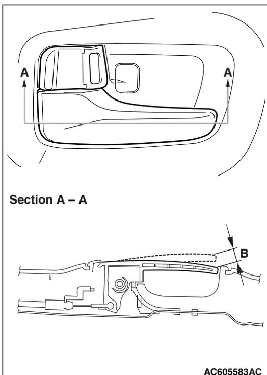
**DOOR INSIDE HANDLE LOCK KNOB STROKE CHECK**
