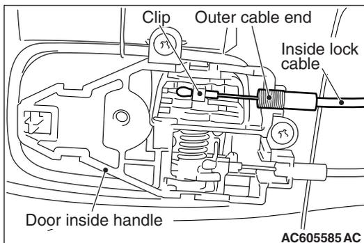
3. If it is outside the standard value, adjust the stroke of the inside handle lock knob by using the outer cable end, which connects the inside handle lock knob to the inside lock cable.
