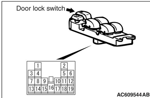
**STEP 3. Check the power window main switch (door lock switch).**
