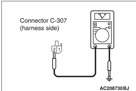
**STEP 8. Check the fusible link (36) line of power supply circuit to the ETACS-ECU. Measure the voltage at ETACS-ECU connector C-307.**
