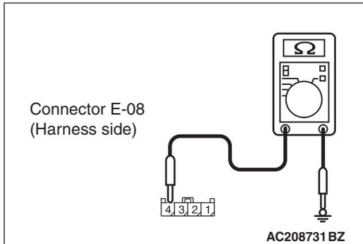
**STEP 10. Check the ground circuit to the front power window sub switch. Measure the resistance at front power window sub switch connector E-08.**
