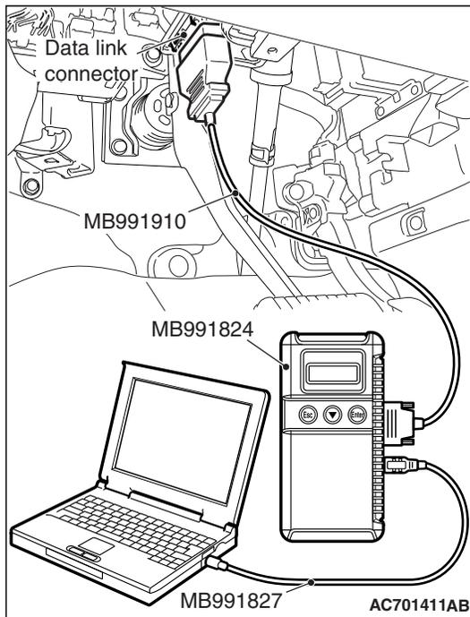
**STEP 4. Using scan tool MB991958, read the diagnostic trouble code.**
