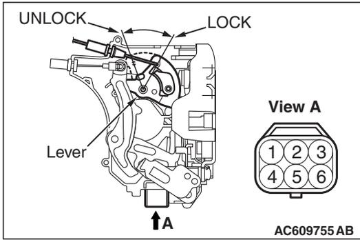
**STEP 11. Check the rear door lock actuator (RH).**
