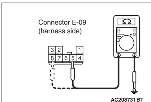
**STEP 11. Check the wiring harness between power window main switch connector E-15 (terminals Nos. 1, 3) and front power window sub switch connector E-09 (terminals Nos. 8, 5).**
