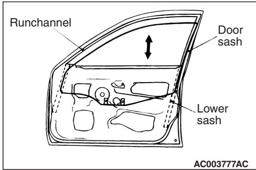
4. If the door window glass does not move up and down smoothly, check and repair as follows:
