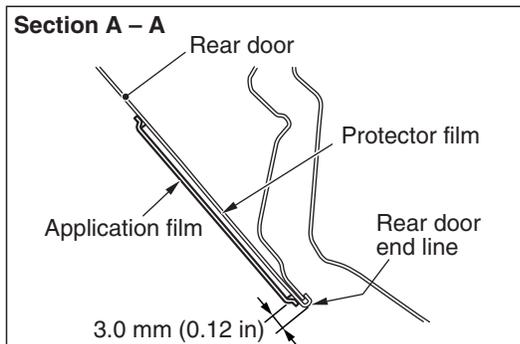
Install the protector film at the position 3.0 mm (0.12 in) away from the rear door end line.
