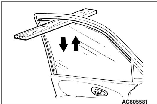
1. Place an approximately 10 mm (0.39 inch) thick wood chip as shown. Then, raise the window glass.
