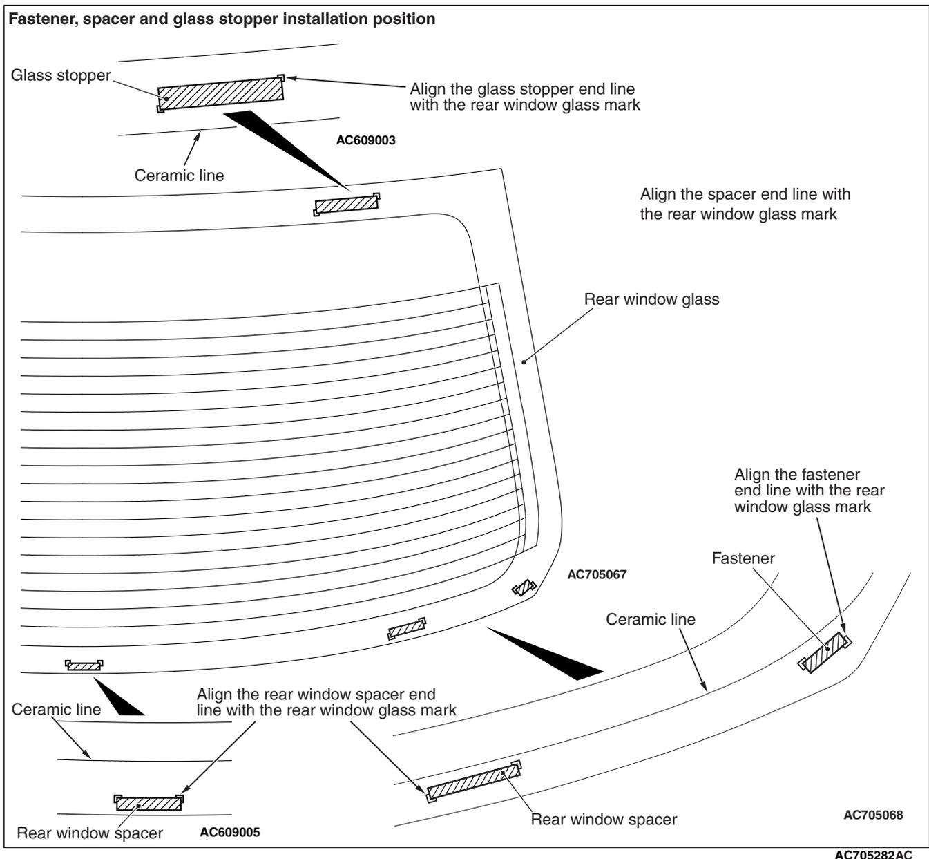
2. Install the fastener, rear window spacers, and glass stoppers to the specified positions so that there are no adrift or warped surfaces inside the rear window glass.
