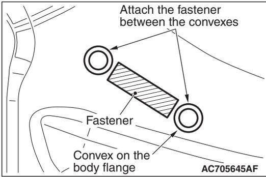
3. Install the fasteners to the specified positions on the body flange.
