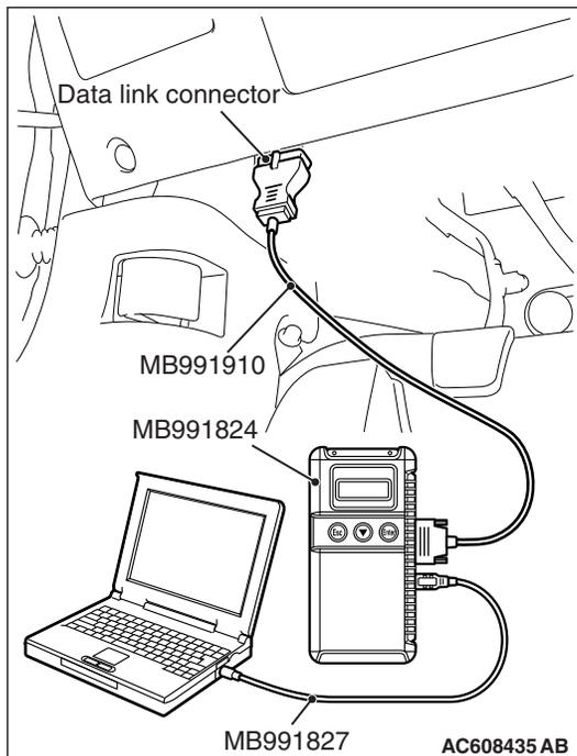
**STEP 2. Register the keyless ID and recheck the diagnostic trouble code.**
