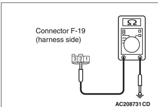
**STEP 6. Check the wiring harness between trunk lid latch connector F-19 (terminal 2) and ground.**
