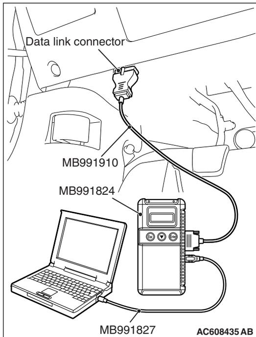
**STEP 2. Using scan tool MB991958, read the occupant classification-ECU diagnostic trouble code.**
