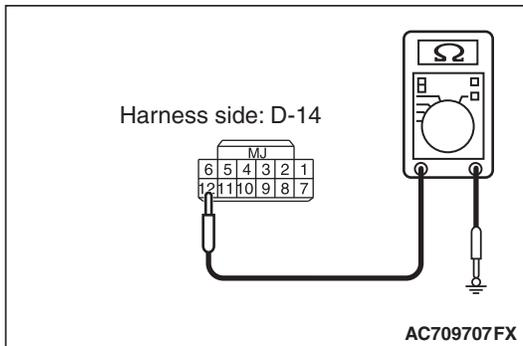
**STEP 4. Check the wiring harness between the receiver antenna assembly connector D-14 (terminal Nos. 8, 12) and the ground for short circuit.**
