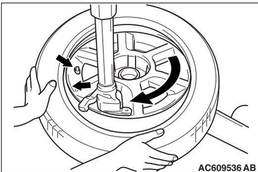
5. Put the second side of the tire in position, so that the cross point of the belt with the rim is approximately 20 cm (7.9 inch) away from the valve. The curved arrow shows the direction of rotation of the wheel.
