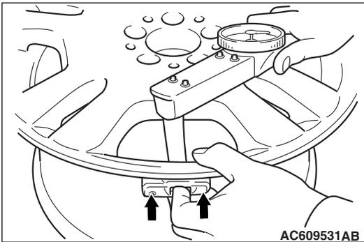
5. While maintaining the TPMS transmitter and valve in position, screw the nut with a torque wrench. Take care that the wrench socket is correctly inserted on the nut.
