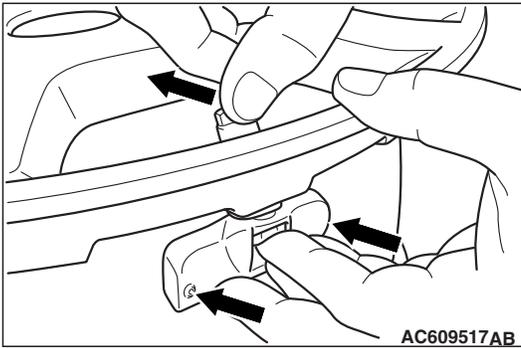
4. While maintaining the TPMS transmitter contact with the rim by applying pressure to the back of the valve, slightly press on the cap to wards the center of the wheel in order to adapt the angle of the valve/TPMS transmitter to the profile of the rim.
