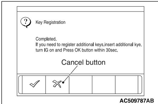
2. When the key registration is completed, "Completed" is displayed. To register the next key, follow the message on the screen and press the OK button. Then, "Executing!" is displayed again and the registration process for the next key starts. To finish the key registration, press the cancel button.
