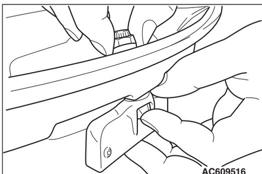
3. When the valve is completely inserted, maintain the TPMS transmitter in contact with the rim, then screw manually the nut until the contact with the wheel.
