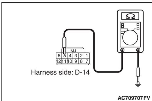
**STEP 8. Check the wiring harness between the receiver antenna assembly connector D-14 (terminal Nos. 1, 3 and 5) and the ground for short circuit.**
