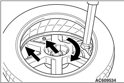
3. Engage the shoe and make sure that 20 cm (7.9 inch) is maintained between the cross point and the valve. The arrow shows the direction of rotation of the wheel.
