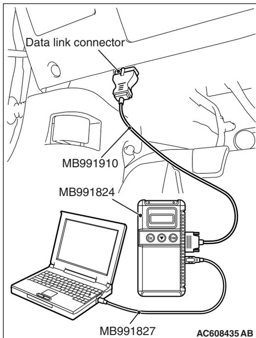
**STEP 2. Using scan tool MB991958, read the A/C diagnostic trouble code**
