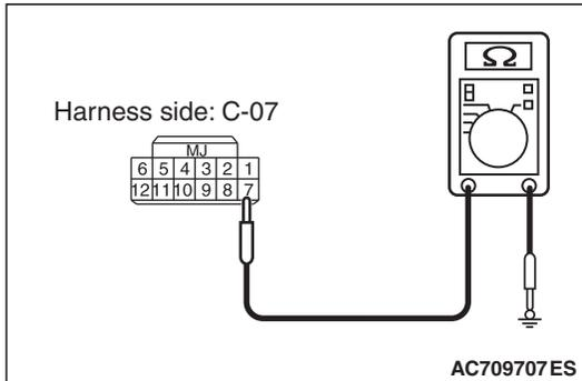
**STEP 3. Check the wiring harness between the WCM connector C-07 (terminal No.7) and the ground for open circuit.**
