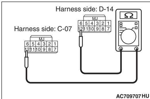
**Q: Is the wiring harness between receiver antenna assembly connector D-14 (terminal Nos. 8, 12) and the WCM connector C-07 (terminal Nos. 8, 12) in good condition?**
