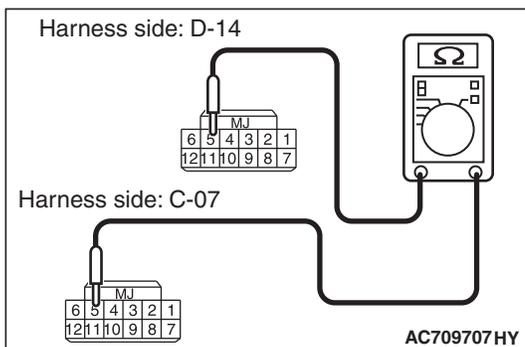
**STEP 7. Check the wiring harness between the receiver antenna assembly connector D-14 (terminal Nos. 1, 3 and 5) and the WCM connector C-07 (terminal Nos. 1, 3 and 5) for open circuit.**
