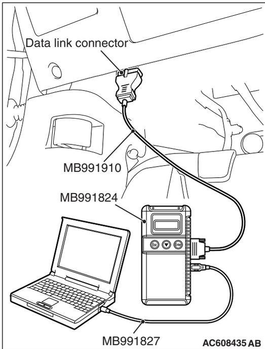
**STEP 2. Register the key ID and recheck the diagnostic trouble code.**
