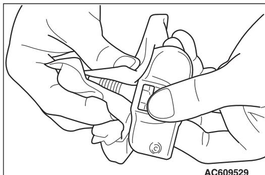
2. Clean the TPMS transmitter and the valve stem holding the valve as shown. Take care to support the rear of the valve with a thumb so that there is no movement of the stem.
