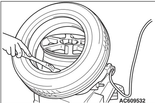
2. Put the tire on the rim, so that the cross point of the belt with the rim is approximately 20 cm (7.9 inch) away from the valve.
