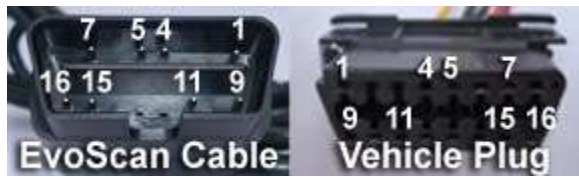
Figure 2. EvoScan OpenPort 2.0 USB Cable pinouts, looking straight-on at the pins on the Cable when its out of the car.
